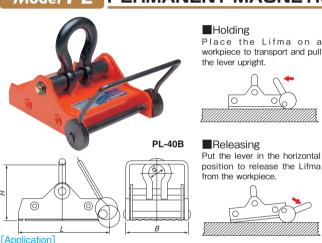
Put the lever in the horizontal position to release the Lifma
