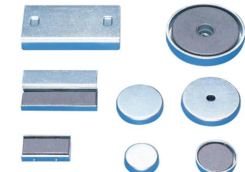
Simple holders consisting of an isotropic ferrite permanent magnet covered by an iron yoke. Dimensionally, the finishing accuracy is not good and these holders are not recommended for incorporation in jigs/fixtures. When these holders are used for the purpose of holding only by themselves, such purpose can be achieved at low cost.
