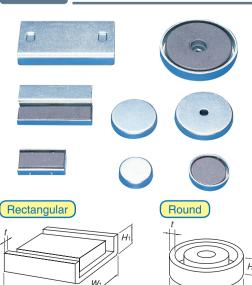
Simple holders consisting of an isotropic ferrite permanent magnet covered by an iron yoke. Dimensionally, the finishing accuracy is not good and these holders are not recommended for incorporation in jigs/fixtures. When these holders are used for the purpose of holding only by themselves, such purpose can be achieved at low cost.
