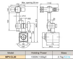
\*The holding power is based on a test piece of SS400, 10 mm thick, ground surface.
