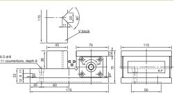
Magnetic force: Side slip resistance is 575 N (57.5 kg) for iron square bars of 30 mm × 30 mm × 130 mm and 480 N (48 kgf) for iron round bars of  $\phi$ 30  $\times$  130 mm thanks to the powerful built-in permanent magnet. Thus, the MAGVICE works well in grinding operations also. Mass: 7.3 kg/ 16.01 lb
