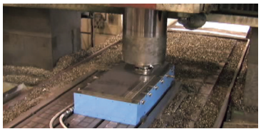
A new construction to prevent occurrence of stick motion failure due to chips employed.
