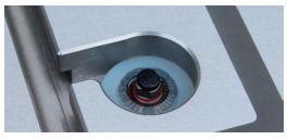
A new construction to prevent occurrence of stick motion failure due to chips employed.
